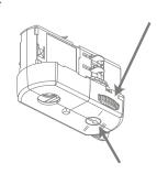
6. Secure the unit to the track by screw
